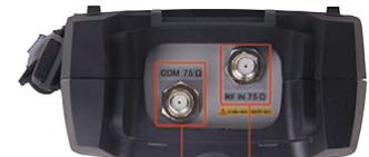
FSK Communication RF Input USG Output
