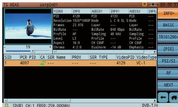
Figure-1 1080p Decoding
