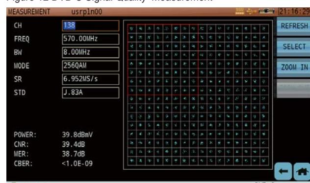
Figure-13 DVB-C Constellation Measurement
