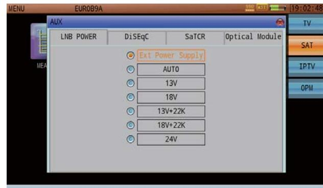
Figure-11 Remote Feeding and Control Signal Setting
