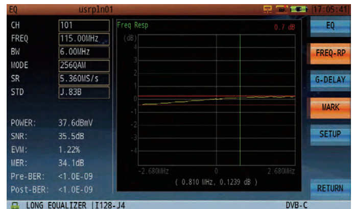
Figure 14: Frequency Response is derived from the adaptive EQ power coefficient. The in-band frequency response should not exceed +/- 1.5 dB peak to valley.
