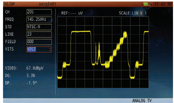
Figure 6: Use VITS and Analog TV Gated Mode to measure analog TV video parameters without interrupting service.
